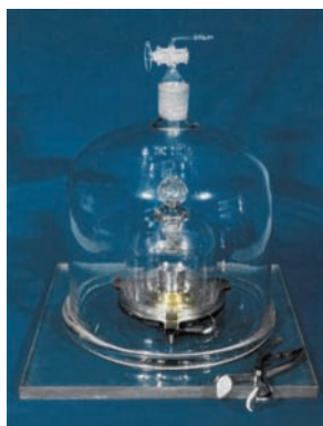
Fig. 3. The prototype kilogram. The only object that has a mass of exactly one kilogram. The prototype kilogram, the last artifact unit of the SI, is kept in a vault at the Bureau International des Poids et Mesures in Sèvres near Paris.
